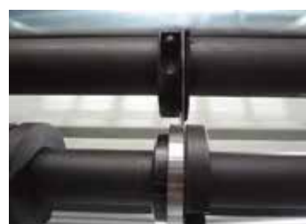
印刷后圆刀分切 Slitter device after printing
