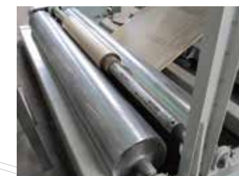
平面收卷 Film central rewinding system
