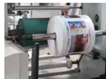
大辊靠背摩擦收卷 Roller friction rewinding system
